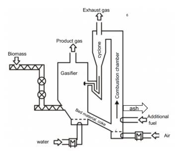
The combustion reaction is used to heat up the bed material which is then circulated back into the gasification bed via a cyclone. The heat of the product gas as well as the exhaust gas from the combustion are used to preheat the fluidization media steam which enters the gasification chamber at 600 °C and air which is needed at 700 °C in the combustion chamber. The 52.2 t/h biomass entering the gasification chamber has a moisture content of 30%. During
